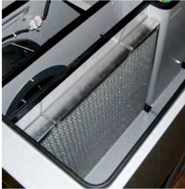
Figure 4-7. Air filter check
