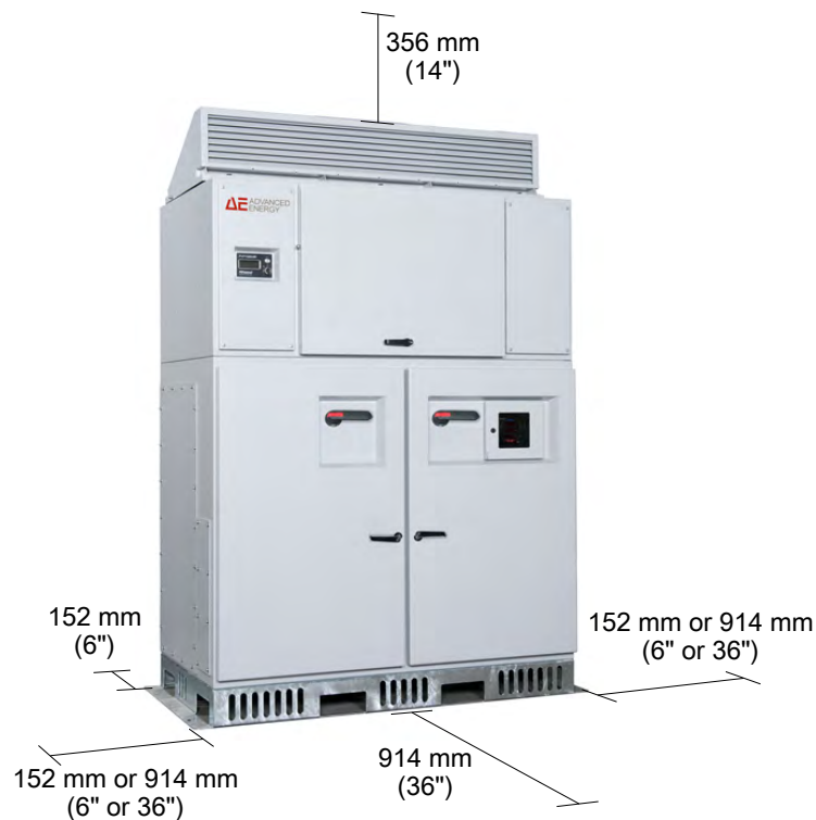
Figure 3-1. Inverter clearances
