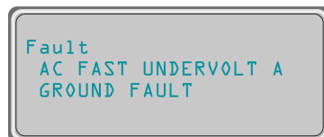
Figure 5-11. Ground fault error message
